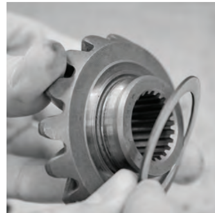
Figure 3-B - MUST REMOVE thrust washers
