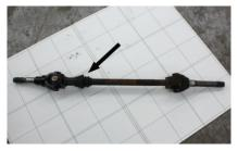
2. In order to install the retaining spring you will need to separate the two axle assemblies at the point indicated.
