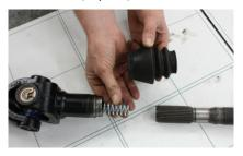
3. Install the retaining spring in between the slip yoke and the intermediate axle.
