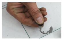
The installation of this carrier assembly does not require the reuse of the factory retaining clip (see above) and has been replaced by the provided axle retaining spring.
