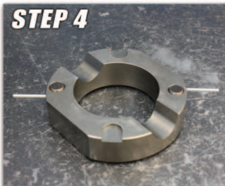
STEP 4 Push alignment pin/spring assembly down & secure with retainer wire
