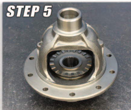
STEP 5 Install side couplers into carrier case
