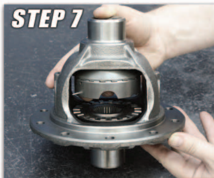
STEP 7 Install center driver & spacers
