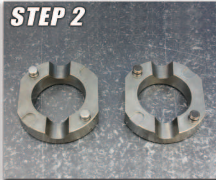
STEP 2 Install alignment pins/springs into driver holes
