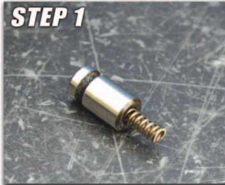
STEP 1 Place springs in hollow end of alignment pins
