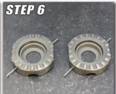
STEP 6 Install spacers into the center drivers
