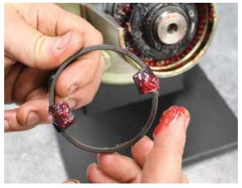
12. Install the Cam Spacer into the retainer plate by aligning the ears on the cam spacer with the notches in the retainer plate.
