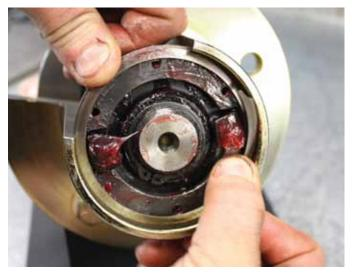
14. Test for proper operation of the cam spacer by compressing the spacer into the hub several times. The cam spacer must freely slide in and out of the hub assembly and return fully seated against the retainer plate. If any binding or resistance occurs disassemble all components and check for proper assembly.
