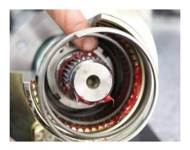
8. Coat the coupler and driver with high pressure grease on all surfaces.
