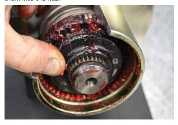
10. While fully compressing the assembly install the axle snap ring if applicable. Assure the snap ring fully seats into the groove on the outer shaft. If no outer snap ring groove exists proceed to the next step in assembly.
