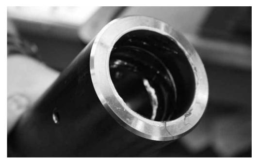
Apply a liberal amount of grease to the boring tool threads.
