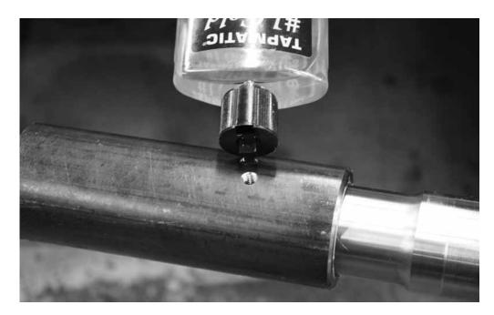
Apply a liberal amount of cutting fluid through the oiling port on the boring tool housing. You will need to add more fluid as you go. It is VERY IMPORTANT to add cutting fluid as necessary to make sure the cutting head has proper lubrication.
