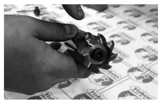
Beging by securing the cutting head and tightening down the bolt.
