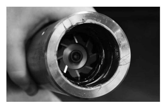
Slide the cutting head/boring shaft into the boring tool housing.
