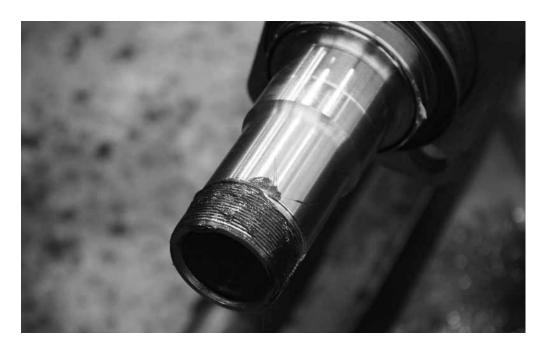
Apply a liberal amount of grease to the spindle threads.
