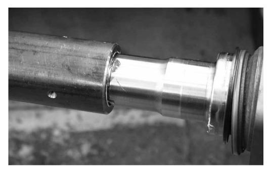
CAREFULLY thread the boring tool into the spindle.
